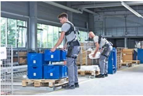
The Paexo Back exoskeleton from Ottobock reduces the strain on the back when lifting heavy objects. (photo: Ottobock)
