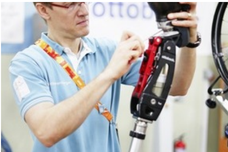
Athletes at the Paralympic Games can come to the Ottobock Repair Service Centers to make sure their equipment is in good shape. The pictures above show O&P professional Peter Schoenenberger servicing a ProCarve sports prosthesis at the 2018 Winter Paralympics in PyeongChang. / © Getty Images for Ottobock
