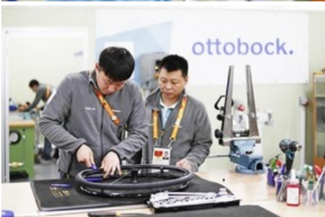
The technical experts on the Ottobock Repair Service Center team also take care of the athletes' everyday devices. This picture shows a tyre change on a wheelchair at the 2018 Winter Paralympics in PyeongChang. / © Getty Images for Ottobock
