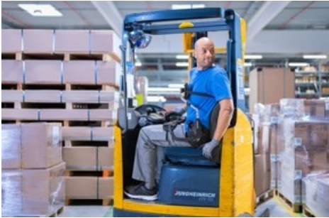
The BackX exoskeleton provides support when lifting heavy loads while also allowing a high degree of freedom of movement, for example when operating a forklift.
