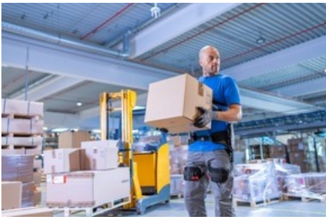
The BackX exoskeleton from Ottobock reduces the load on the user's back by up to 13kg during lifting.
